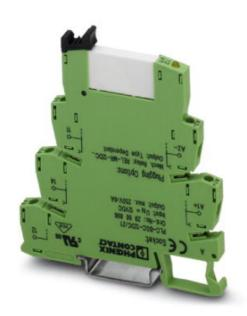
PLC relay, consisting of base terminal block PLC-BSC.../21 with screw connection and pluggable miniature relay with power contact, for assembly on mounting rail NS 35/7.5, 1 PDT, input voltage 12 V DC
